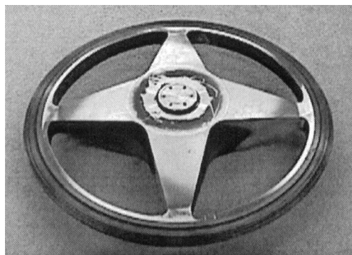
Figure 11. Burst flywheel rotor with machined outer diameter.
